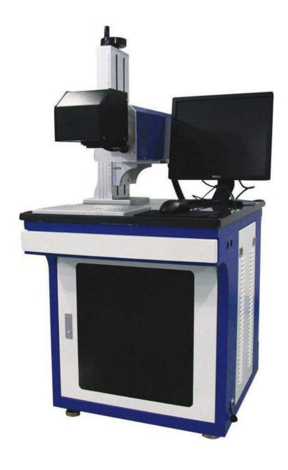
Integrates advanced galvanometer laser marking technology with imported well-known excited sealed CO2 laser, makes it more amazing for non-metal materials marking, it's one of the most popular laser marking machines in domestic and overseas markets.
